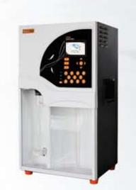
Automatic accurate distribute alkali and boric acid solution
