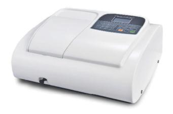
The 5600 and 5800 series include 4 models: V-5600, UV-5600, V-5800 and UV-5800. They all have a Lead screw structure which ensures high wavelength accuracy of the instrument. 5800 series with more accurate technical specifications in several beautiful for the series of the series o ification is your best choice for sin-gle beam spectrophotometer.
