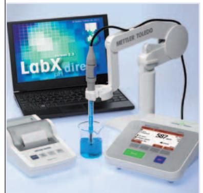
Upon endpointing SevenCompact™ allows multiple archiving options: the data can be stored, printed or transferred to LabX direct. Any combination of these three options is possible giving you total flexibility.
