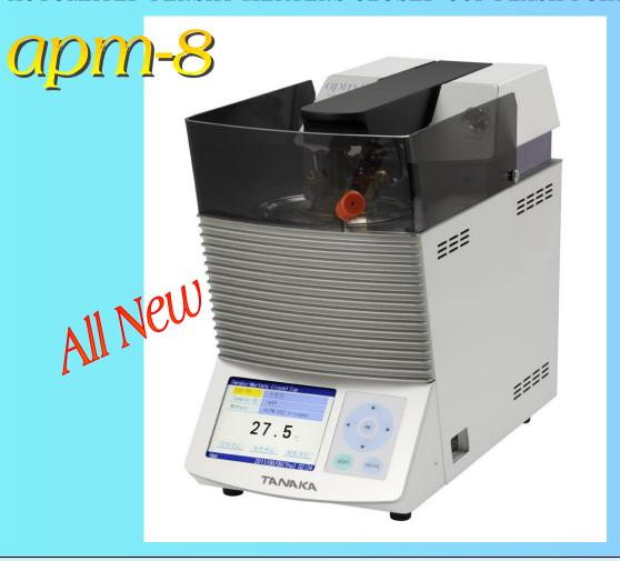
Model apm-8 is the automated Pensky-Martens Closed Cup flash point tester from Tanaka. Based on 45 years experience of manufacturing the automated flash point testers, innovative 8th generation series has been released. The theme of 8th generation is "Ergonomic, Versatile and Premium".
