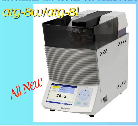
Model atg-8 series is the automated Tag Closed Cup flash point tester from Tanaka. Based on 45 years experience of manufacturing the automated flash point testers, innovative 8<sup>th</sup> generation series has been released. The theme of 8<sup>th</sup> generation is "Ergonomic, Versatile and Premium".
